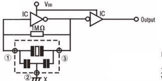
IC(MG,MT):1/6TC4069UBPx2 (MX) :1/6TC74HCU04x2 X: Ceramic Resonator VDD: +5V
